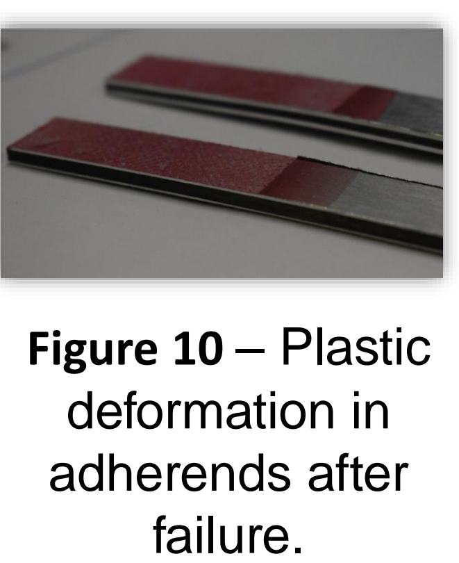
Figure 8 – Failure mode of SLJ's with highrate loading.
